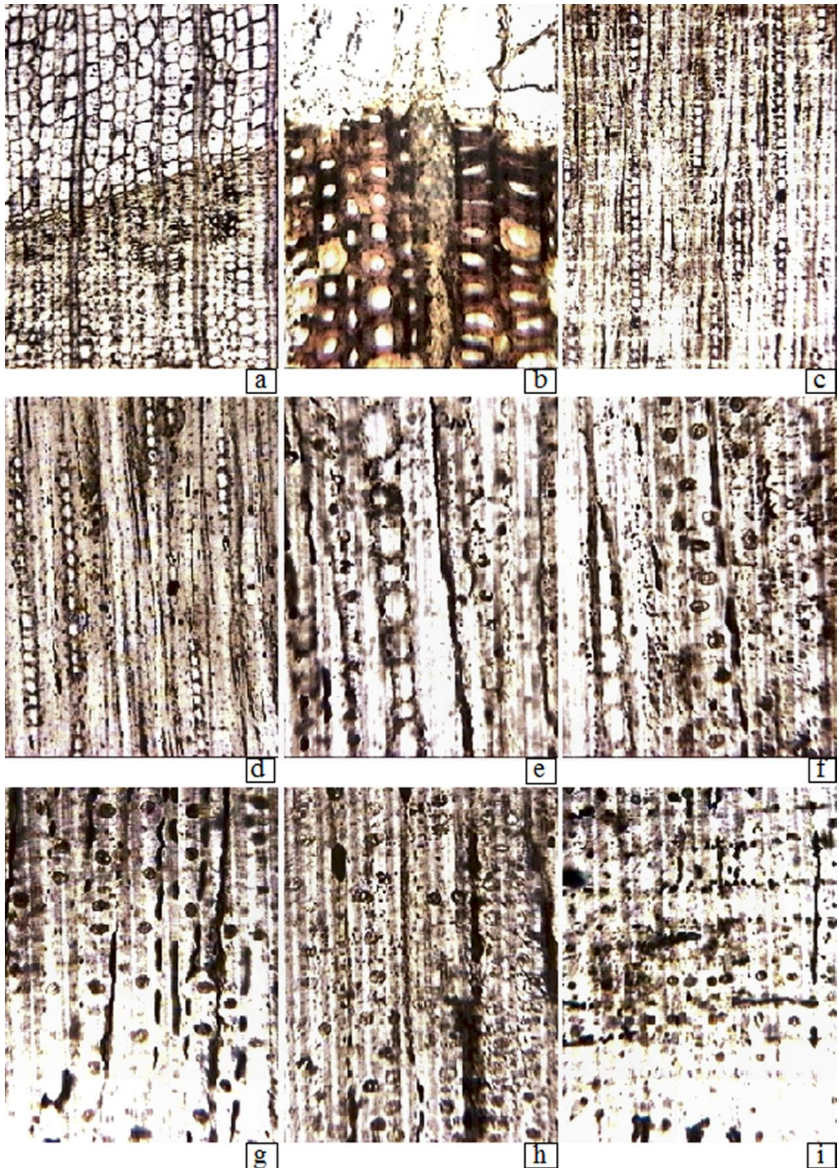
Fig. 5 Thujoxylon sp. a, b - cross section: distinct growth-ring boundary, linear rays, very thick-walled tracheids in late-wood - x100-x200; c, d - tangential section: high uniseriate rays - x100; e, f - tangential section: rare small tangential pits on tracheids - x200; g, h - radial section: uniseriate spaced pitting - x200; i - radial section: cross-field pitting - x200.
